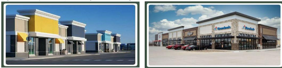
Figure 26.03 The buildings in the above images contain pilasters, cornices, and a series of facade setbacks (recesses) to visually break up the appearance of large facades.
